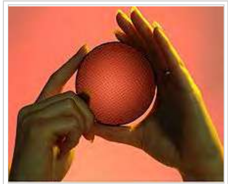
Low-temperature oxidation catalyst used to convert carbon monoxide to less toxic carbon dioxide at room temperature. It can also remove formaldehyde from the air.
