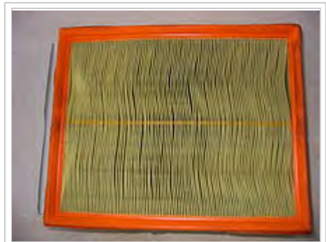
Used auto engine air filter, clean side
