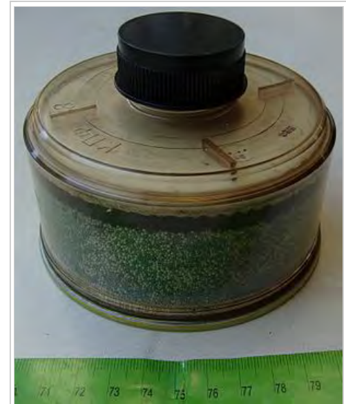
Combined gas and particulate respirator filter for protection against acid gases, the type of BKF (БКФ). It has transparent body and special sorbent that changes color after the saturation. This color change may be used for timely replacement of respirators' filters (like End of Service Life Indicator ESLI).
