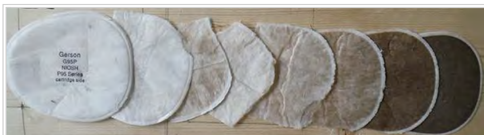
Cross-section of a disposable NIOSH P95 filter pad used in metalworking operations. Even "clean" industrial processes often generate large amounts of harmful particulate matter and require breathing protection.
