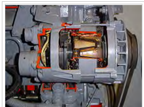
Cut-away of an alternator, showing the claw-pole construction; two of the wedge-shaped field poles, alternating N and S, are visible in the centre and the stationary armature winding is visible at the top and bottom of the opening. The belt and pulley at the right hand end drives the alternator.
