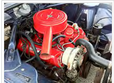
Alternator (silver) mounted on a V8 engine
