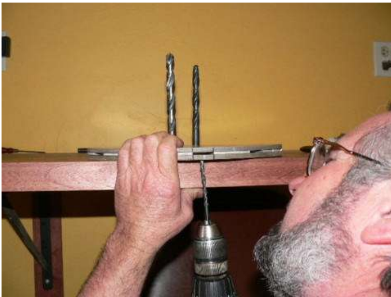
(drilling into the bottom magnet rotor)
