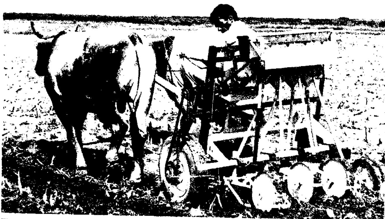
Fig. 4-10: Mekins Nikart with fertilizer-planter (Photo: ICRISAT archives).
