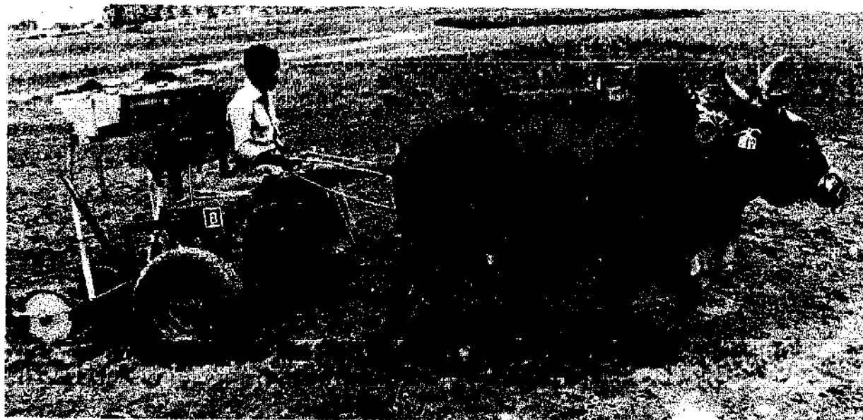
Fig. 2-16: Designed in 1962, modified by ICRISAT, and promoted worldwide, the Tropicutor spans all phases of development. Here seen with seeder and fertilizer distributor at ICRISAT Centre, 1985. (Photo: P.H. Starkey).
