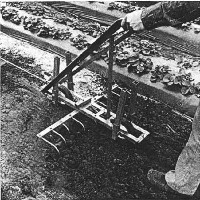
Figure 3-22 A specially designed, multiuse frame with a cultivator attachment to harness the full potential of the winch
