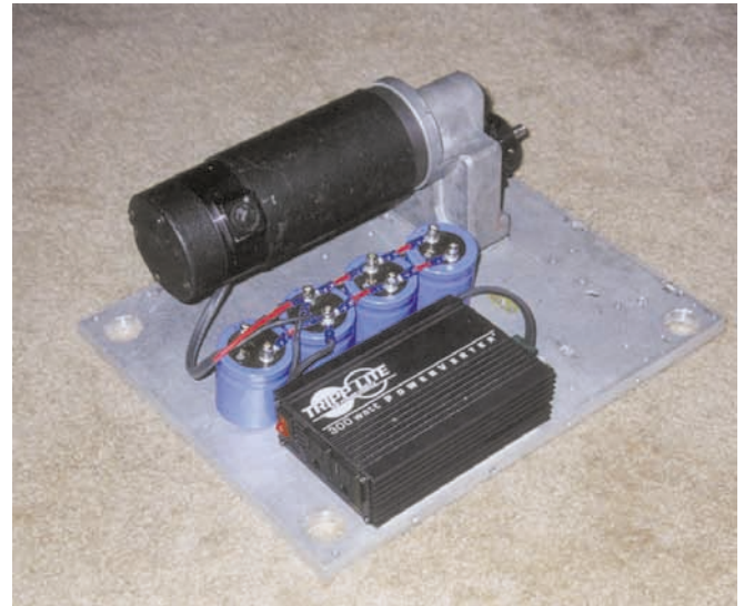
Generator #3, capacitors, and inverter mounted and ready to install. A 1/2 inch (13 mm) thick aluminum plate serves as the base. The generator is bolted on while the capacitors and inverter are held on with Velcro.
