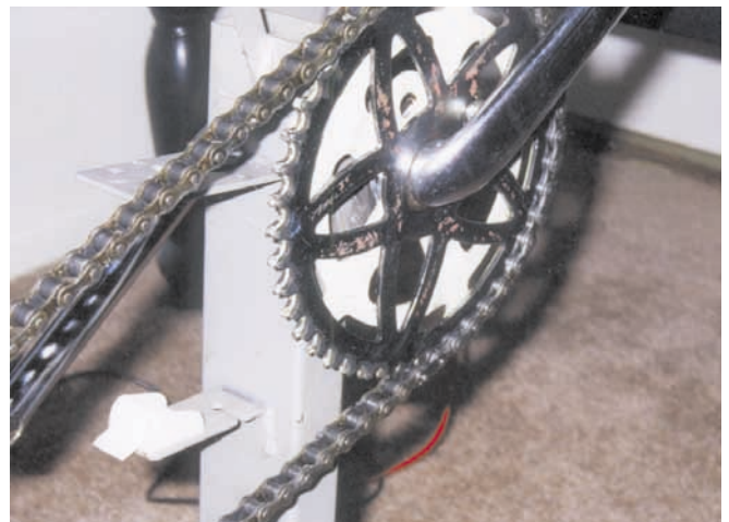
Close-up of the side-by-side sprockets. The white sprocket is behind the chrome sprocket.
