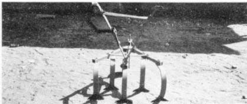
Figure 37: The Houe Manga in this illustration has the four left-hand tines correctly aligned. The right-hand tine, however, needs adjusting.
