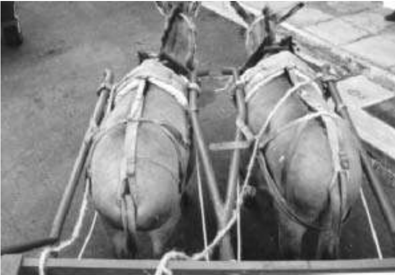
Figure 24: Four-shaft design for hitching two donkeys with collar and saddle to a two-wheeled cart (photo: Luurt Oudman).
