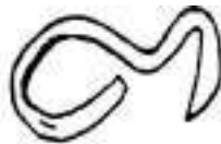
Figure 8: A hoof pick can be easily made by bending a piece of round steel into the desired shape with one end flat and pointed.
