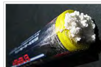
Leaked alkaline battery
