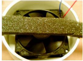
Round the corers of the fan and cut a piece of foam about .75 by .75" by 14" long.
