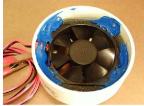
Hold it in place with a bit of silicon rubber II gasket sealer.
