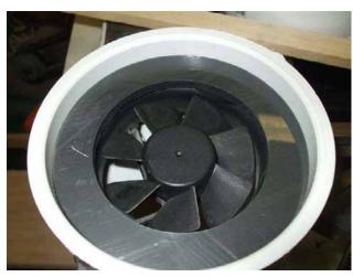
This method has an advantage if one uses a one way flow flapper valve. This would be a thin sheet of plastic hinged to open when the fan is running and gravity would close it when the fan is not running.
