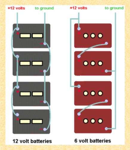
When replacing your batteries, remove the negative cable first because this will minimize the possibility of
