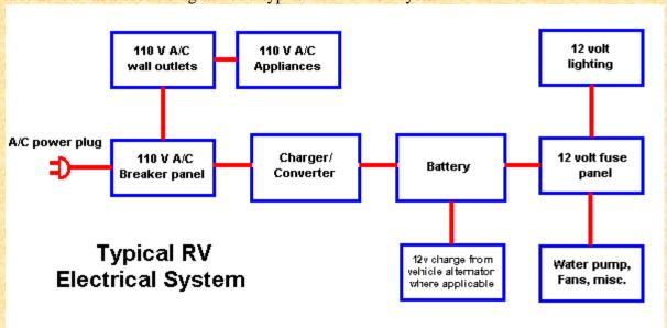
See.. there's really nothing to it! In the simplest terms, you have lights and other equipment such as water pump, fans, stereo, etc. that run on 12 volts, a battery that supplies the 12 volt power and some sort of charger to replenish the energy that you use from the battery. Of course, it's possible to add lots of useful components to this simple system to make it more flexible, but the basic 12 volt system in any RV starts with the components shown above.
