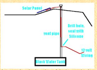
Once inside the RV, the wire can be routed to the location of the battery bank and connected to the charge controller.
