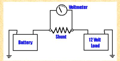
We will be using the same panel voltmeter as above to build our amp meter. Some basic wiring ingenuity and the use of a suitable switch will allow you to use a single panel meter for both functions... more on that later. First, the shunt must be built or purchased. You will need a .01 ohm shunt, one that's rated 10 mvolt / amp. Shunts are available from a variety of sources, but you can also build your own! I constructed mine from a set of
