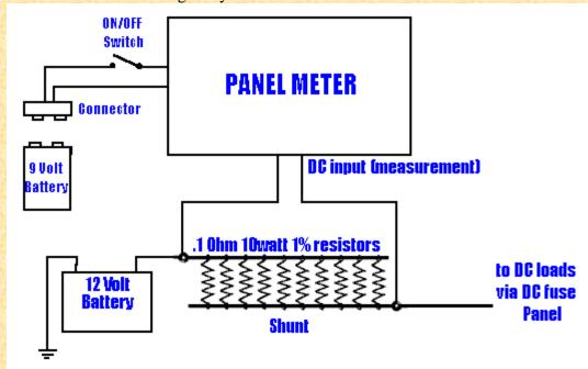
Here's a wiring diagram that I used to build my volt/amp meter for my rig. This allows you to use the one panel meter to monitor both amps and volts.
