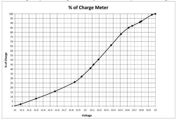
A typical car battery has about 40-80 amp-hr fully charged or about 1 amp-hr/pound of battery. A typical deep cell battery has about 100-200 amp-hr fully charged or about 2 amp-hr/pound. By weight one can estimate the maximum capacity.
