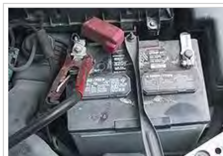
A positive (red) jumper cable connected to battery post. An optional hydrometer window is visible by the single jumper clamp. (The black negative jumper clamp is not shown.)
