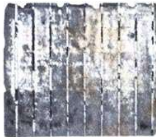
Fig. 36—Severely-notched separator due to vibration of loose element, or battery loose in cradle.
