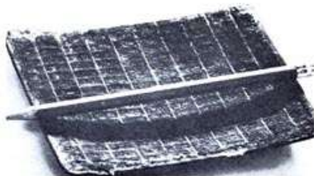
Fig. 33—Severely buckled Positive Plate.
