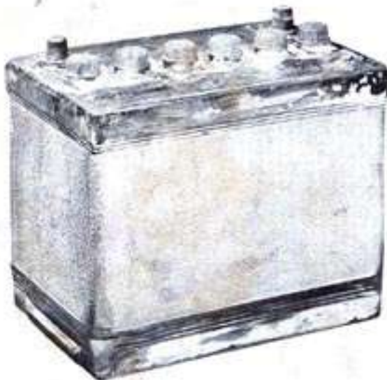
Fig. 37—Container worn by loose hold-downs.
