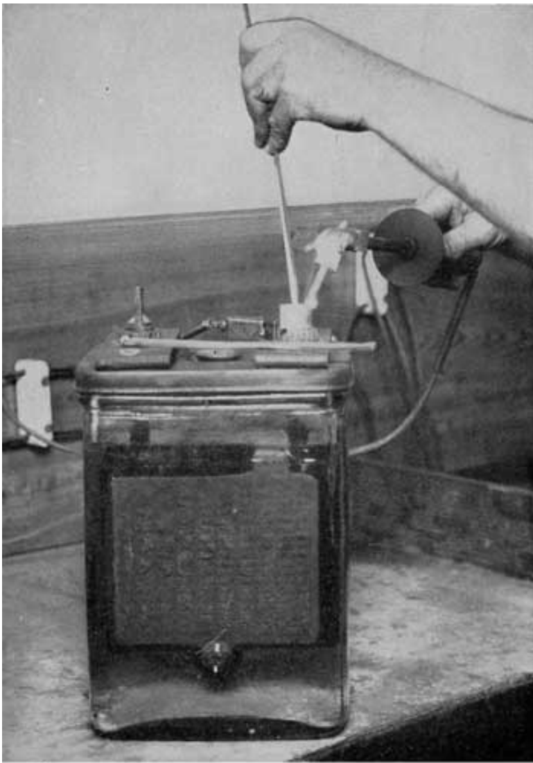
Fig. 319. Burning on Negative Strap. Delco-Light Cell
