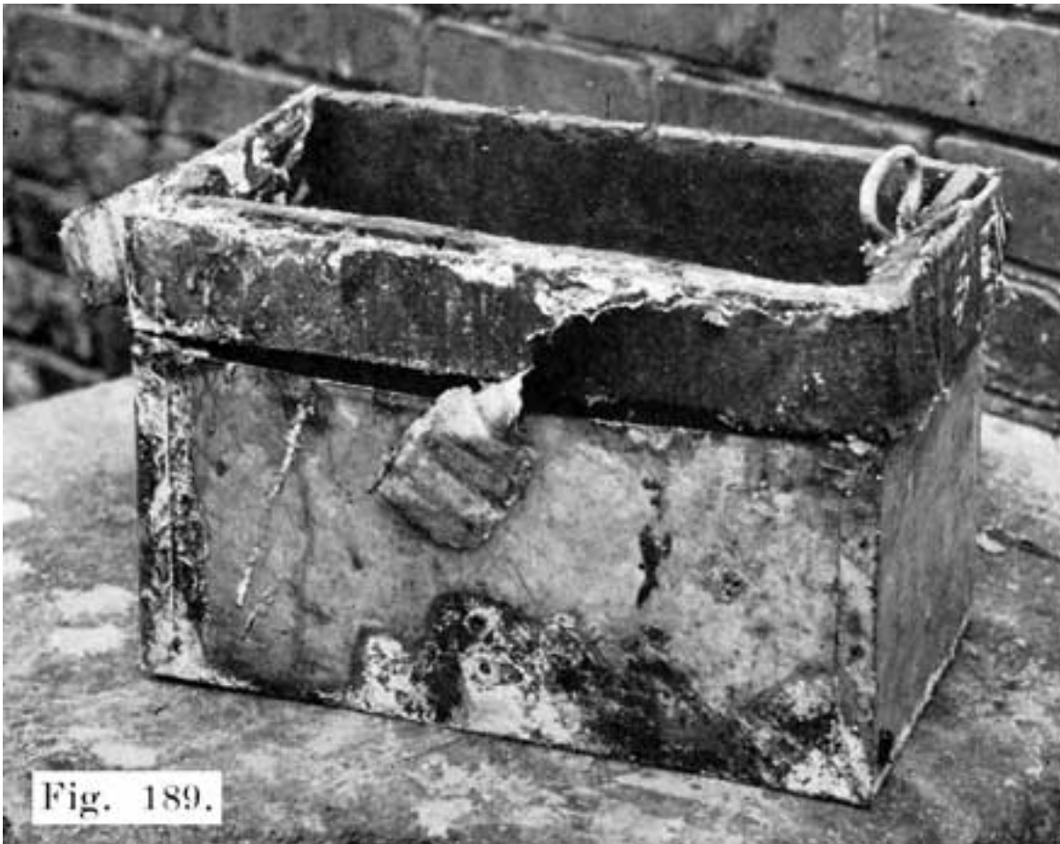
Fig. 189. A Blacksmith and Tinsmith Tried Their Hands on This Case, Lower Part Enclosed in Tin, Strap Iron, Covered with Friction Tape, Around The Top.
