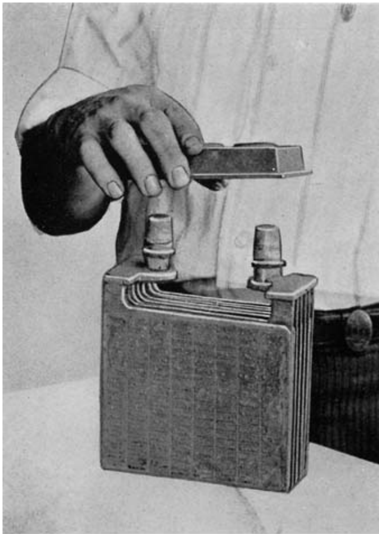
Fig. 252. Replacing Prest-O-Lite Cover on Built Up Posts
