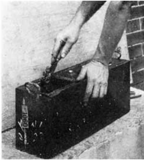
Fig. 200. Removing Compound from Top of Jar
