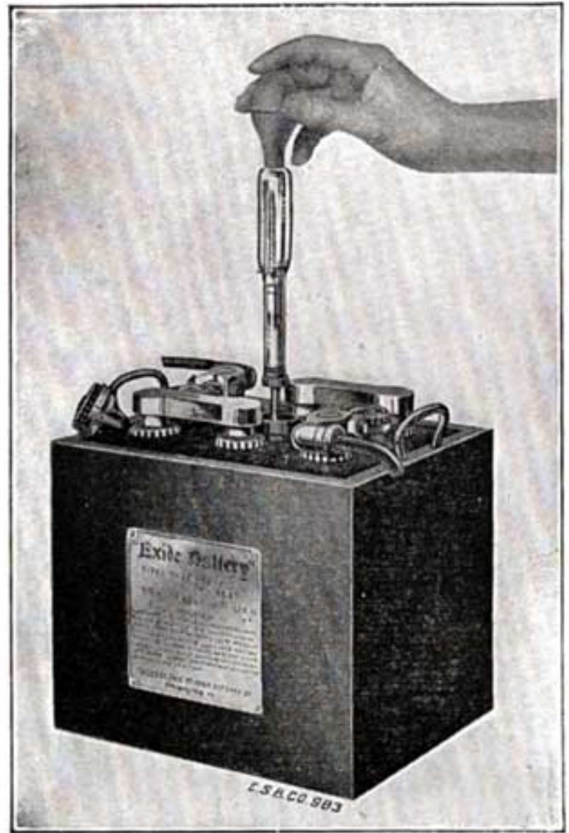
Fig. 35. Taking a Specific Gravity Reading
