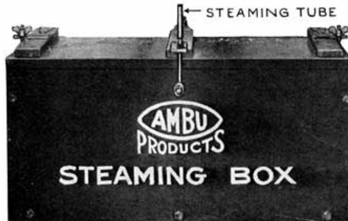
Fig. 93. Steaming Box in Which Entire Battery is Set
