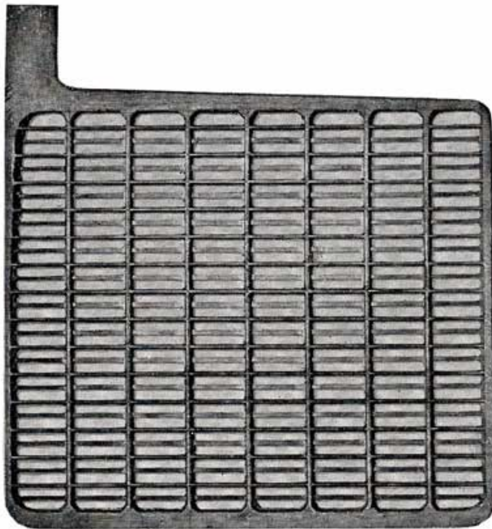
Fig. 4. Grid, Trimmed, and Ready for Pasting
