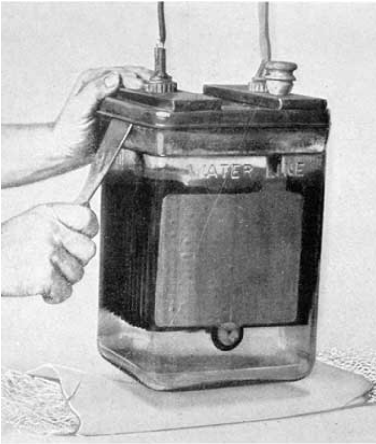
Fig. 306. Removing Delco-Light Cell Cover
