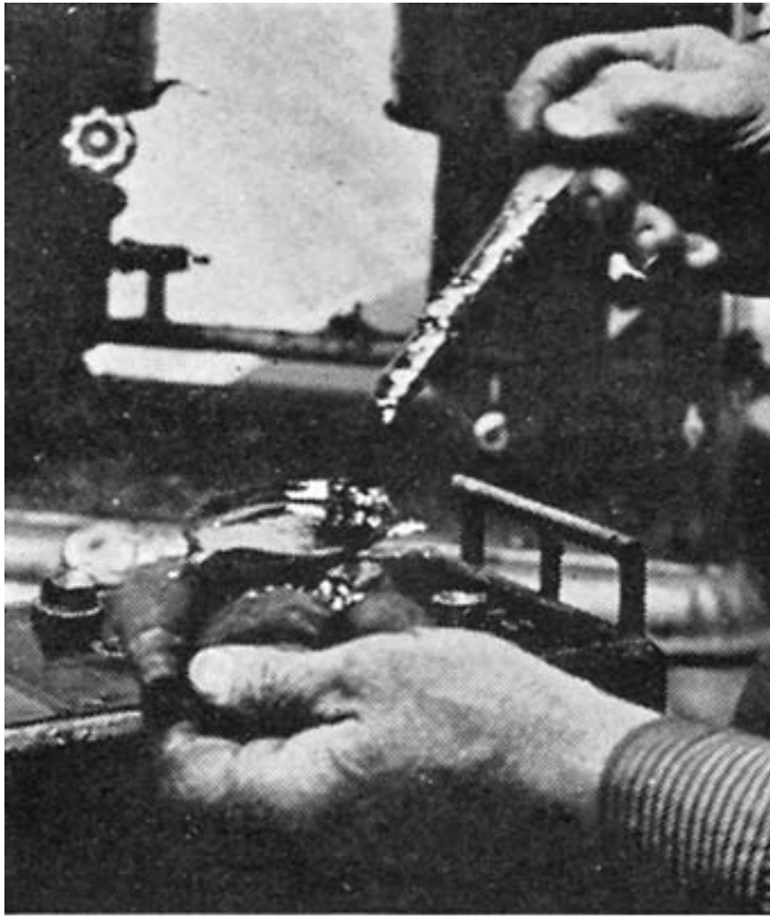
Fig. 235. Wiping Bottom of Spoon Filled with Seal- ing Compound
