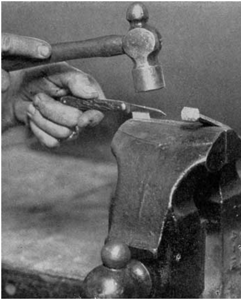
Fig. 318. Splitting End of Strap. Delco-Light Cell
