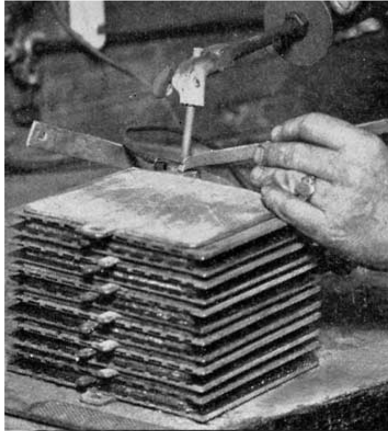
Fig. 322. Burning on Outside Negative Plate. Delco-Light Cell
