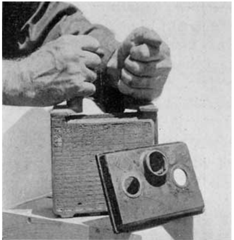
Fig. 227. Shifting Groups to Make Cover Fit
