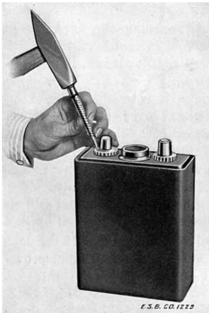
Fig. 241. Upsetting Threads to Prevent Nut from Turning
