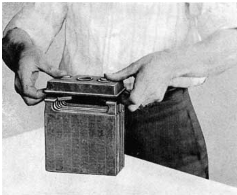
Fig. 250. Removing Prest-O-Lite Cover
