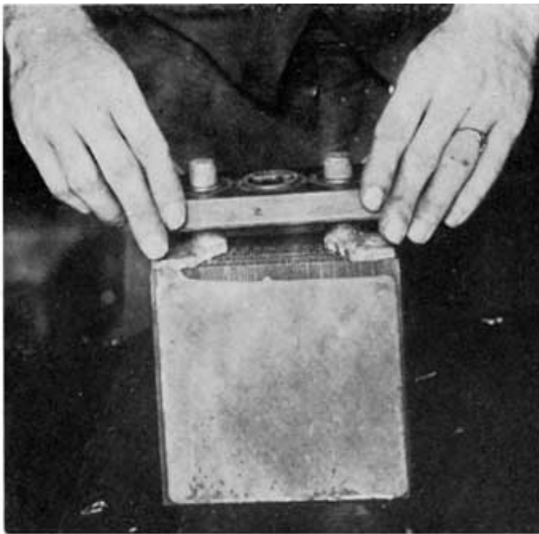
Fig. 258. Replacing Cover of Philadelphia Diamond Grid Battery
