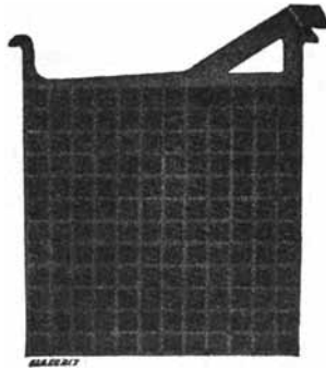
FIG. VII. BOX NEGATIVE PLATE.
