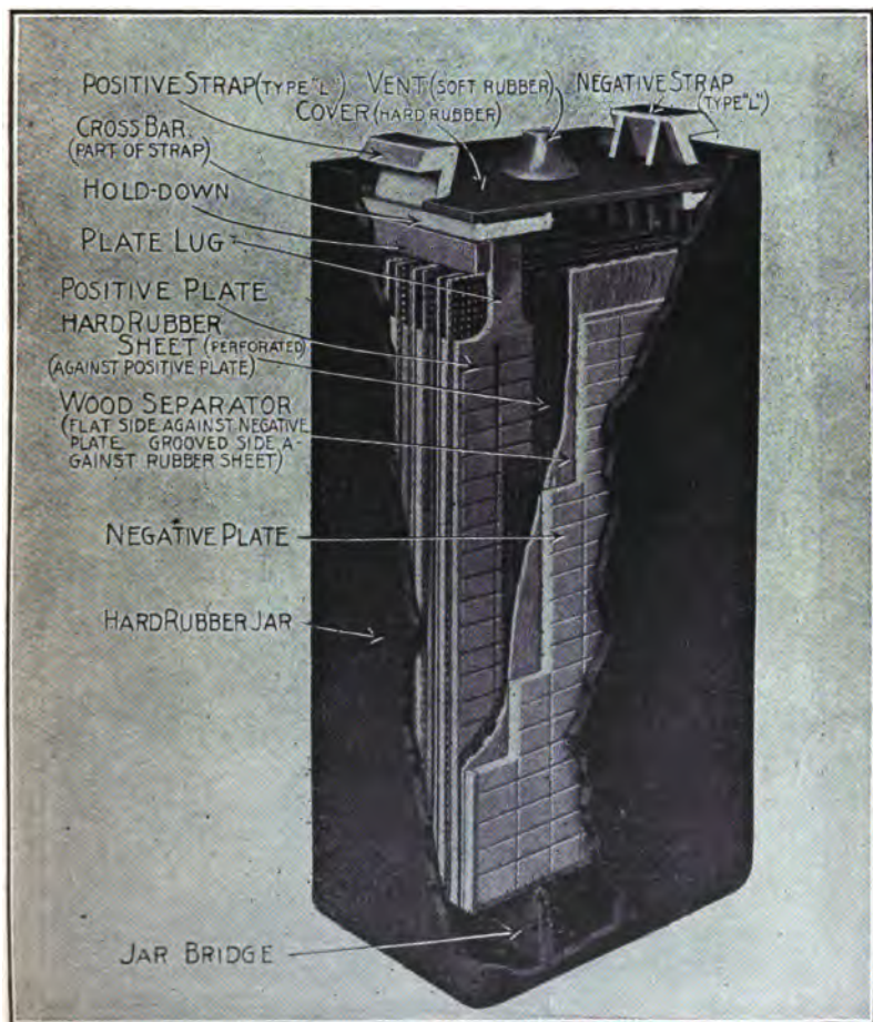
Fig. 16.—Part Sectional View of Gould Pasted Plate Cell.
