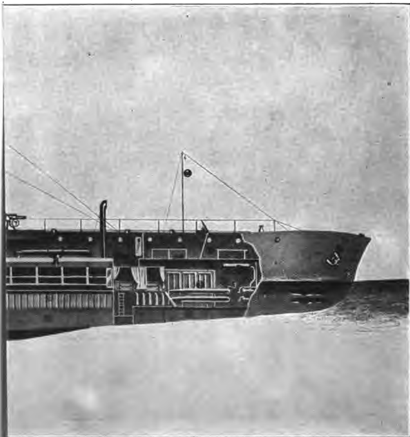
Drop Keel. 5—Habitable Superstructure. 6—Escape and Safety Hatches. 12—Torpedo Firing Tank. 13—Anchor. 14—Periscopes. 15—Storage Battery. 22—Galley. 23—Steering Gear. 24—Binnacle. 25—Engines. 31—After Engine-Room and Engines. 32—Cannery Room. 38—Hydroplane. 39—Vertical Rudders. 40—Signal
