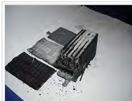
Disassembled AGM battery. From left: positive plate, glass mat separator, negative plate. On the right are the five remaining cells (of the six-cell battery).
