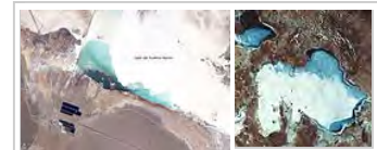
Satellite images of the Salar del Hombre Muerto, Argentina (left), and Uyuni, Bolivia (right), salt flats that are rich in lithium. The lithium-rich brine is concentrated by pumping it into solar evaporation ponds (visible in the left image).
