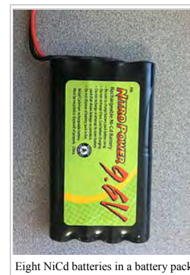
Eight NiCd batteries in a battery pack
