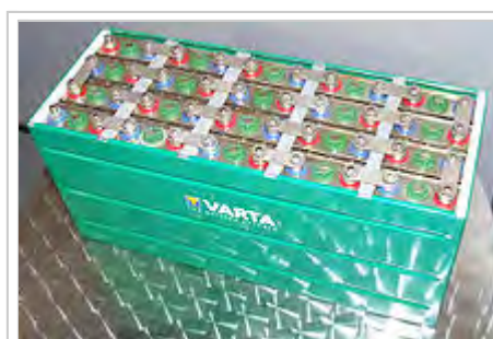
Nickel–metal hydride 24V battery pack made by VARTA, Museum Autovision, Altlusheim, Germany
