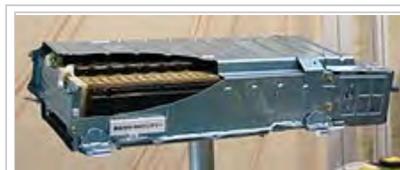
High power Ni–MH battery of Toyota NHW20 Prius, Japan
