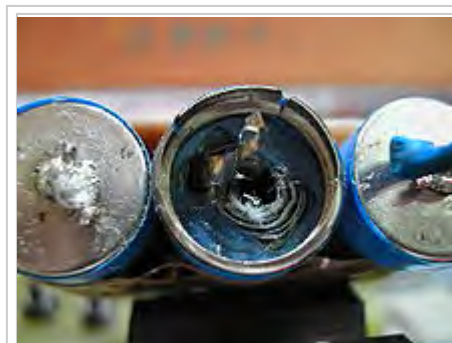
NiMH cell that popped its cap due to failed safety valve
