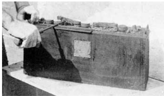
Fig. 193. Prying Off Cell Connector
