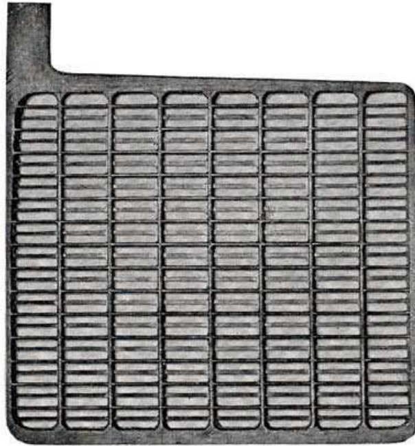
Fig. 4. Grid, Trimmed, and Ready for Pasting
