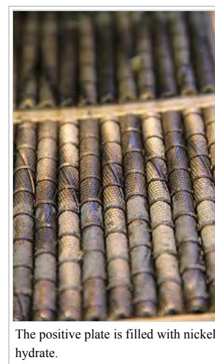
The elements of a nickel iron (NiFe) cell
