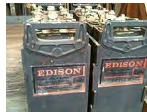
Nickel–iron batteries manufactured between 1972 and 1975 under the "Exide" brand originally developed in 1901 by Thomas Edison.
