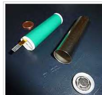
Cylindrical cell (18650) prior to assembly. Several thousand of them (lithium ion) form the Tesla Model S battery (see Gigafactory).
