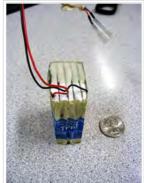
Side-view of water-activated radiosonde battery
