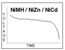
and then suddenly plummet. This contrasts to alkalines, which lose their capacity steadily. For this reason many electronic devices that tell you how much battery life is left have a hard time reporting an accurate level for rechargeables, but this is especially true for NiZn's, because their voltage is so high.
