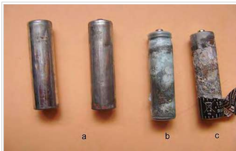
Progressive corrosion of zinc–carbon batteries.
