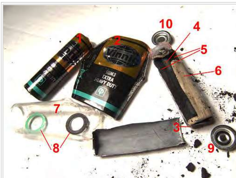
Disassembled zinc chloride cell (similar to zinc carbon cell). 1:entire cell, 2:steel casing, 3:zinc negative electrode, 4:carbon rod, 5:positive electrode (Manganese dioxide mixed with carbon powder and electrolyte), 6:paper separator, 7:polyethylene leak proof isolation, 8:sealing rings, 9-negative terminal, 10-positive terminal (originally connected to carbon rod)
