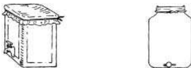
Figure 31: Container made from a petrol tin, for filling jars (left) and a plastic container with tap (right).
