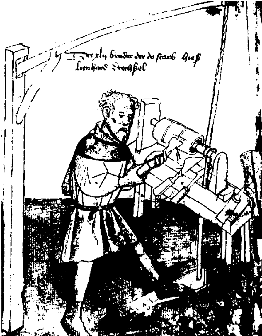
Figure 1-18 Foot-powered lathe (Courtesy of Friedrich Klemm)
