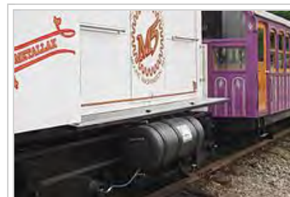
Biodiesel locomotive and its external fuel tank at Mount Washington Cog Railway
