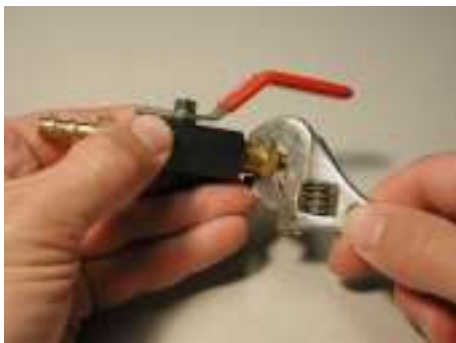
Installing the barb fittings on the ball valve.
