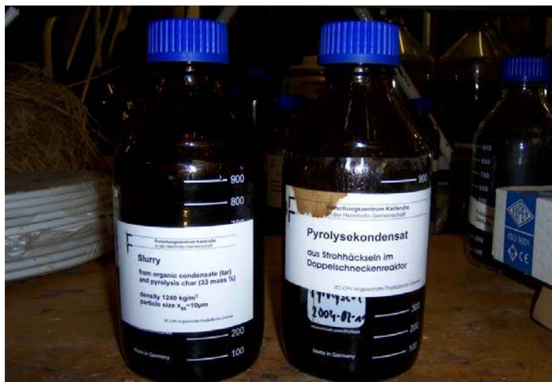
Figure 40: Slurry produced with the bioliq process
