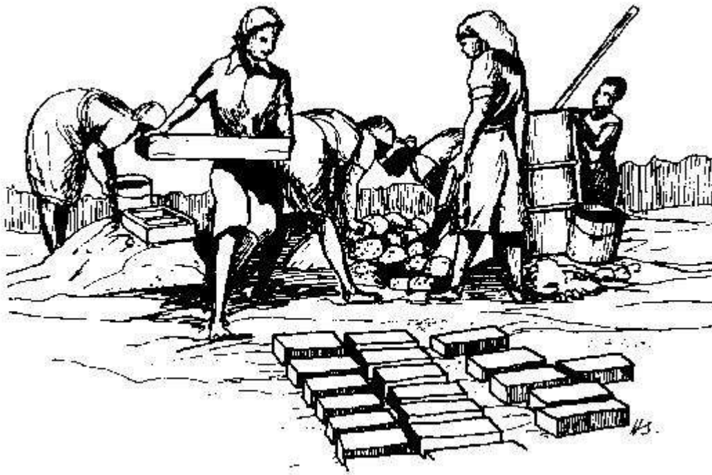
A self-help group of women in Zimbabwe making bricks for building latrines.
