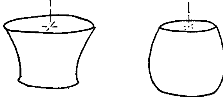
Fig. 4 curved walls are stronger than flat walls
