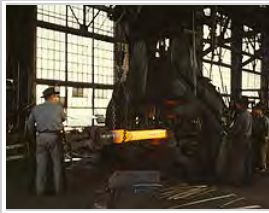
Hammering out a draw bar on the steam drop hammer in the blacksmith shop, Santa Fe Railroad shops, Albuquerque, NM, 1943.
