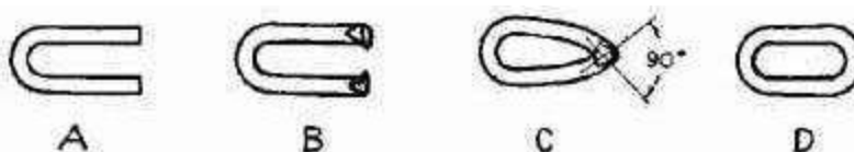
FIG. 269.—Steps in making a link.
