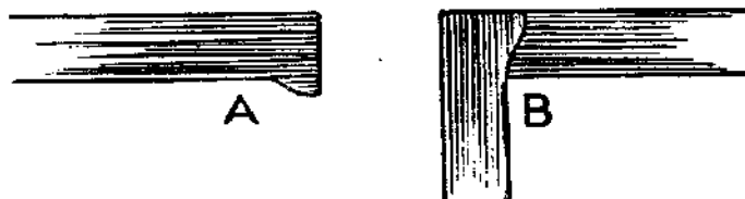
FIG. 28. WELDING FLAT IRONS AT RIGHT ANGLES
