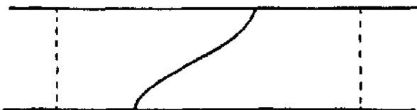
FIG. 42. HOW TWO SHORT LANDSIDES MAY BE CUT FROM A 9-INCH LENGTH OF STEEL
