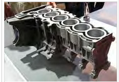
An engine block with aluminium and magnesium die castings.
