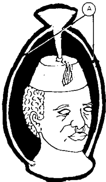
Fig. 38 The addition of runners. A The runners.
