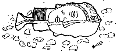
Fig. 5 Shattering the mould to release the cast bust.
