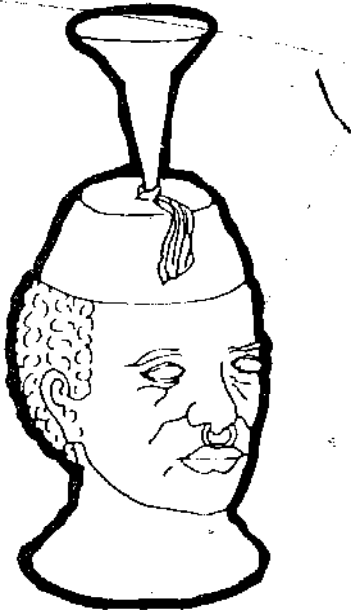
Fig. 37 A wax pattern with sprue and pouring cup.
