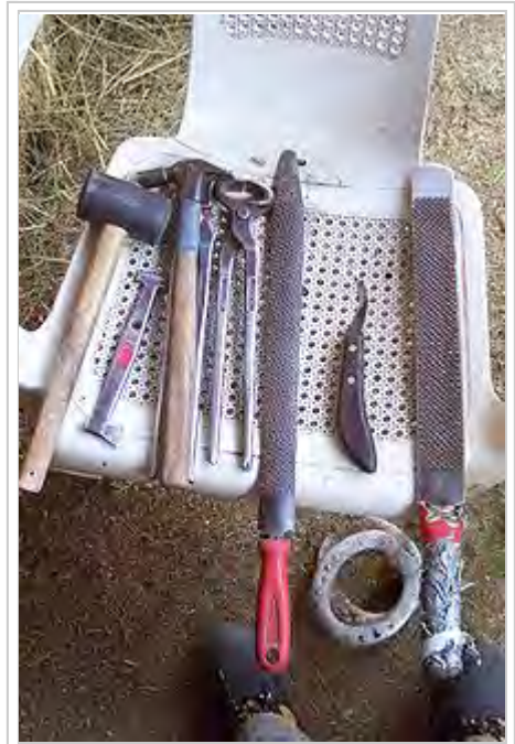
Some farrier tools, including hammers, nippers, rasps, and hoof knife, a set of custom-made corrective shoes are shown below the toolset
