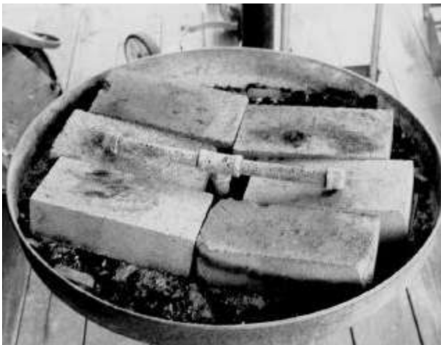
Placement of the bottom bricks and tuyere
