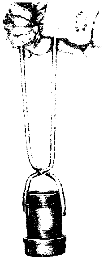
TONGS GRIP crucible securely when removing it from furnace for pouring molten metal in molding flask
