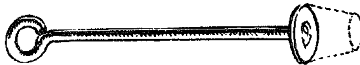
Fig. 91. A "bot" stick with a dotted indication of the shape of the "bot."
