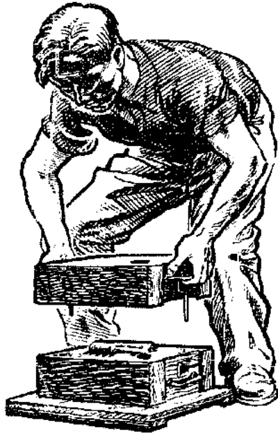
Fig. 21. Closing a large mould.
