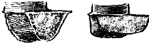
Fig. 85. Two sections of iron runners. The right is free from chill. The left bears evidence of chilling.
