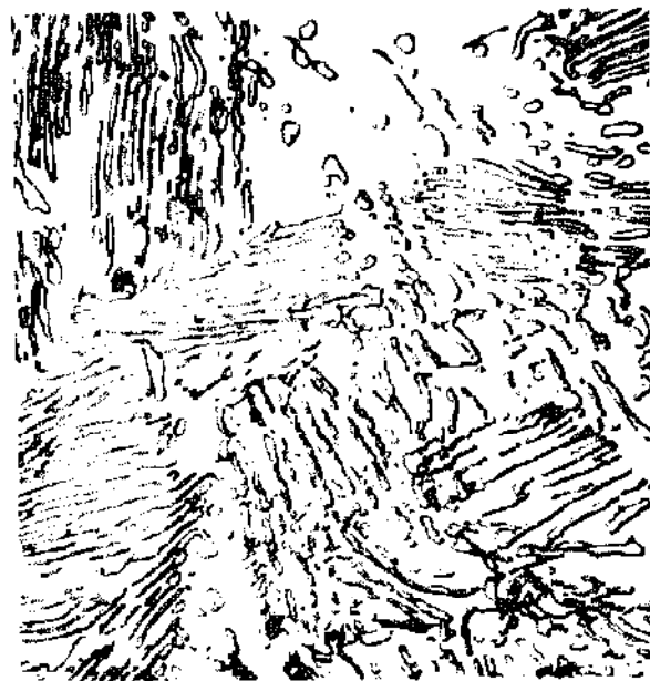
Fig. 15-12. Photomicrograph of an iron-carbon alloy made by mixing iron and graphite powders, pressed at 50 tsi (689,500 kN/m 2 or 689.5 MN) and sintered at 2100°F (1177°C) for 30 minutes. Shows a pearlitic structure similar to that of annealed carbon tool steel. Magnified 1000 times.
