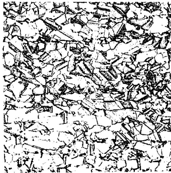
Fig. 18-13. Aluminum-silicon bronze, extruded. Aluminum 7 percent; silicon 2 percent; copper balance. Alpha plus beta structures. (Revere Copper and Brass, Inc.)
