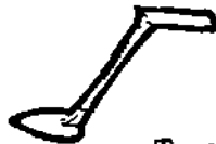
Trowels for cutting sand
