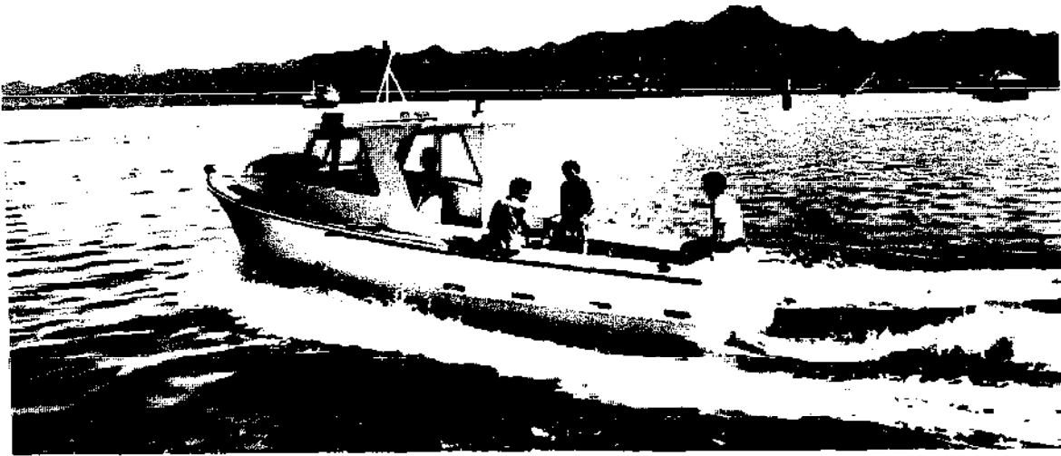
Fig. 7. Boat built from Fig. 3 design, running at 12 knots at design trim.
