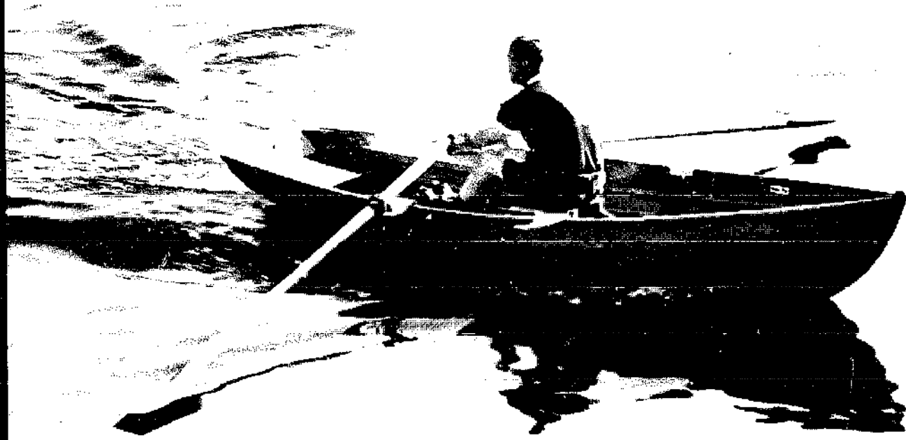
Above: A 13-foot Chamberlain dory skiff built by Thomas G. Plant, Jr., of San Francisco. This rowing model is fitted with a sliding seat and spoon blade oars. Below: The same model dory skiff built by Plant and rigged for sail.
