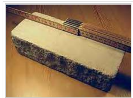
Swedish Mexitegel is a sand-lime or lime-cement brick.
