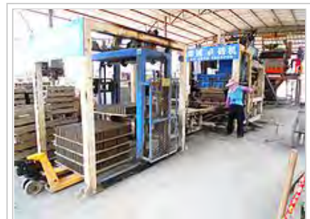
A concrete brick-making assembly line in Guilinyang Town, Hainan, China. This operation produces a pallet containing 42 bricks, approximately every 30 seconds.
