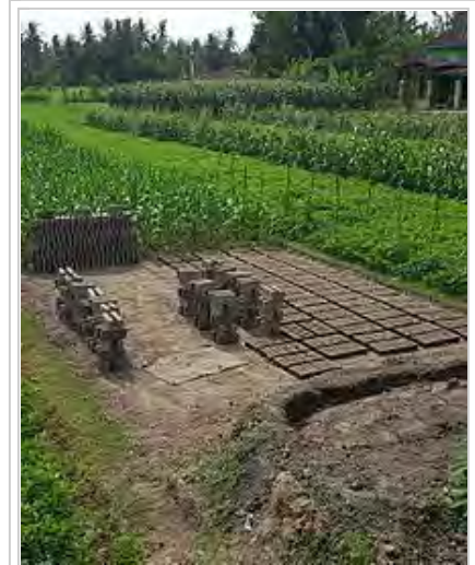
Raw bricks were sun-dried before fired
