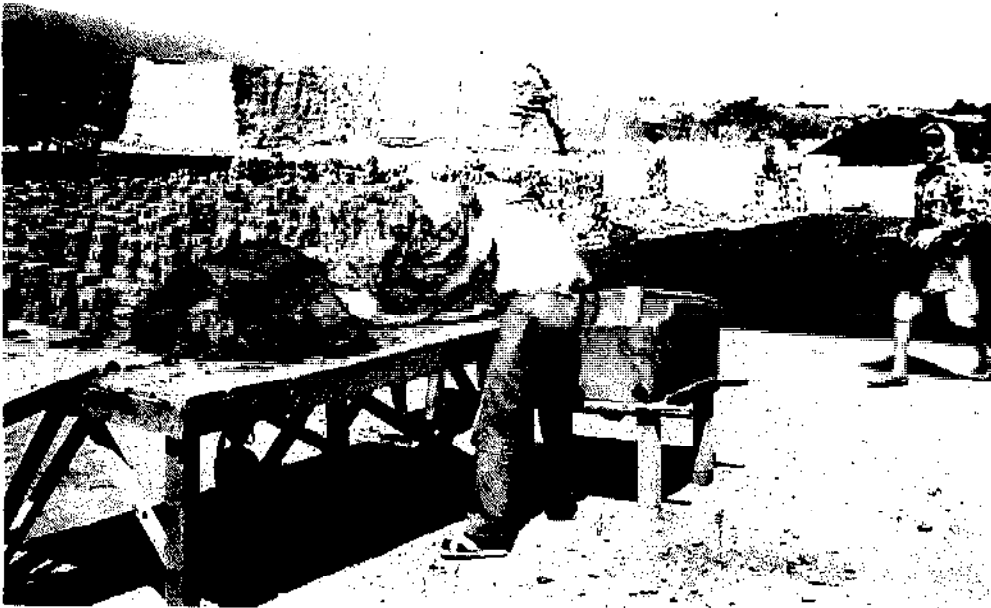
Moulders filling three-compartment moulds at table and setting bricks out on open air drying floor
