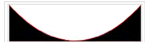
Comparison of a catenary (black dotted curve) and a parabola (red solid curve) with the same span and sag. The catenary represents the profile of a simple suspension bridge, or the cable of a suspended-deck suspension bridge on which its deck and hangers have negligible mass compared to its cable. The parabola represents the profile of the cable of a suspended-deck suspension bridge on which its cable and hangers have negligible mass compared to its deck.
