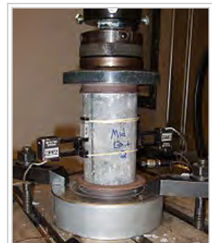
Compression testing of a concrete cylinder
