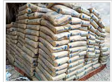
A few tons of bagged cement. This amount represents about two minutes of output from a 10,000 ton per day cement kiln.
